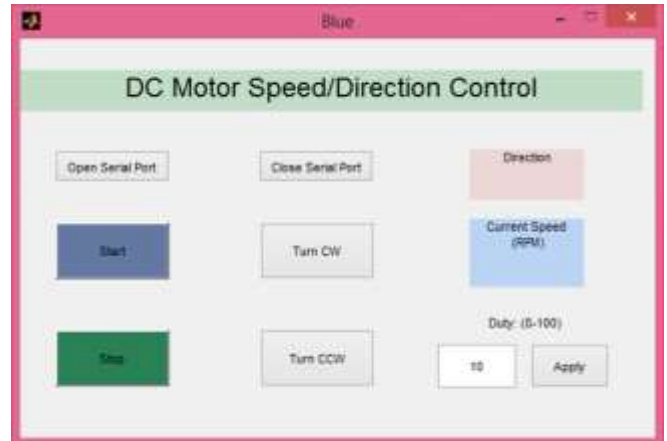
Figure 4. Speed and position controller user interface of DC motor with wireless communication
