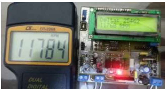
Figure 6. Measurement results with application circuit and digital tachometer
