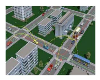
Fig. VANET in a city scenario. Vehicles are warned of the truck blocking the road, and alternate routes [6]
