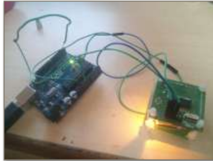
Fig: 2.1 : Arduino (Left) interfaced with the RFID reader (Right)
