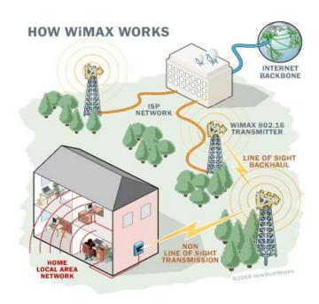
Several topology and backhauling options are to be supported on the WiMAX base stations: wireline backhauling (typically over Ethernet), microwave Point-to-Point connection, as well as WiMAX backhaul. With the latter option, the base station has the capability to backhaul itself. This can be achieved by reserving part of the bandwidth normally used for the end-user traffic and using it for backhauling
