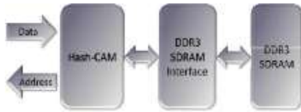
Figure 1: Hash-CAM lookup circuit using DDR3 SDRAMs
