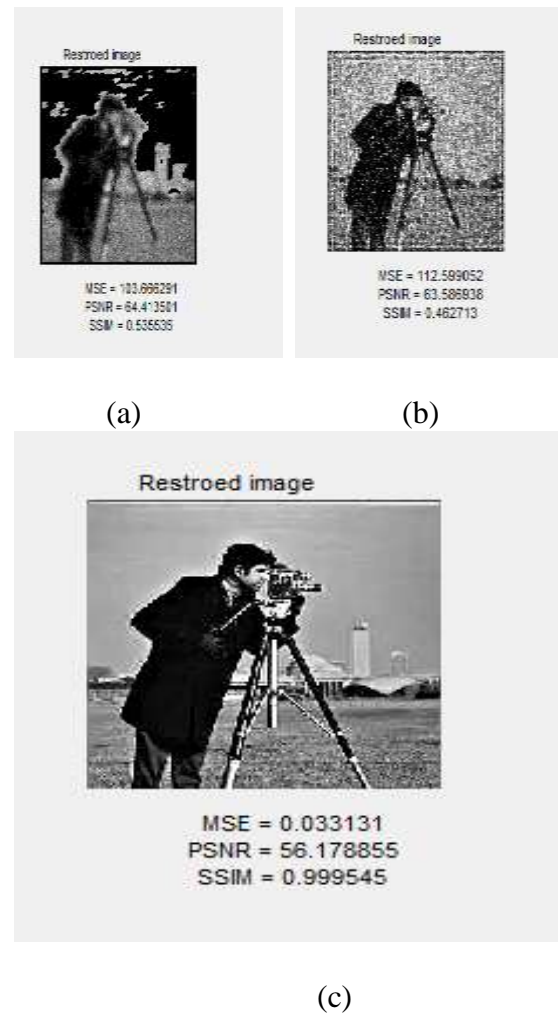
Fig 4 Restored Image using Blind Deconvolution Method (a) MLE Algorithm (b)EM Algorithm (c) MAP Algorithm
