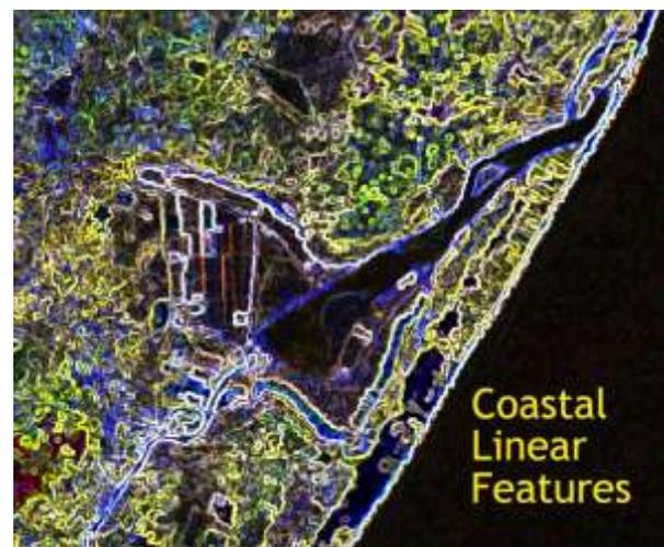
Figure 4. Linear feature and boundary detection in coastal area using Sobel filter
