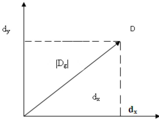
Figure 1. Image gradients using vector geometry
