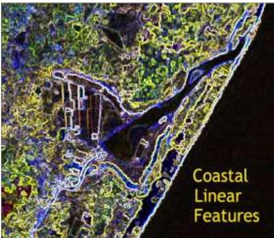
Figure 5. Linear feature and boundary detection in coastal area using Prewitt filter
