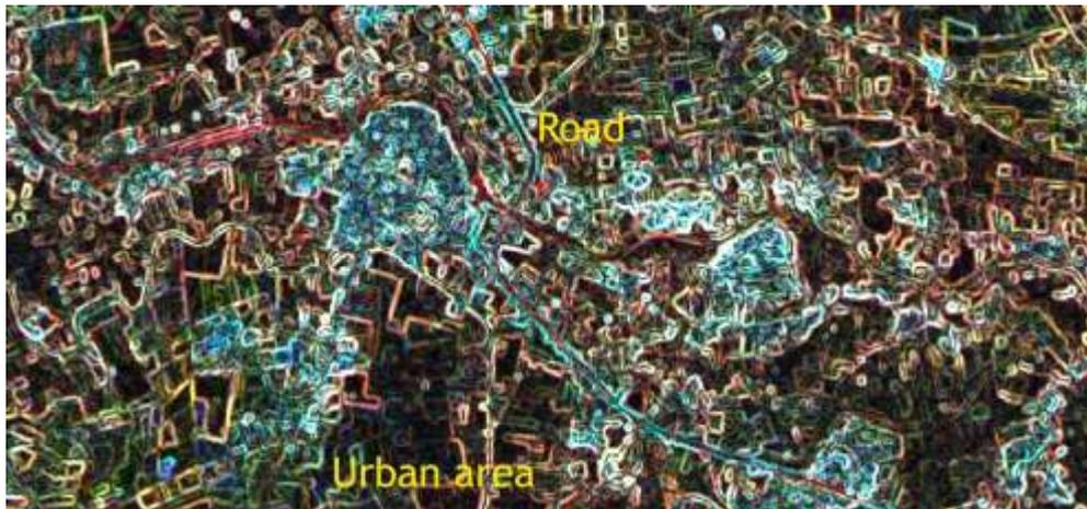
Figure 2. Linear feature and boundary detection in an urban area using Sobel filter
