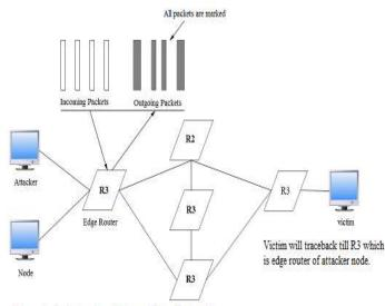
Edge router in attack path will take part in traceback to the attacker node.Packets will be marked at edge router.
