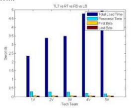
**Figure 18**: Total Load time, Response time, first byte, last byte of Tech Team website
