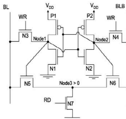
Fig3: 9T SRAM cell.
