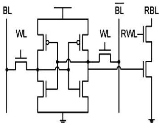
fig2: 8T SRAM cell
