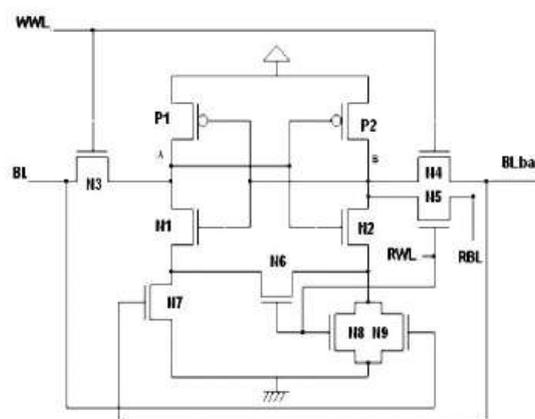
Fig4: 11T SRAM cell.
