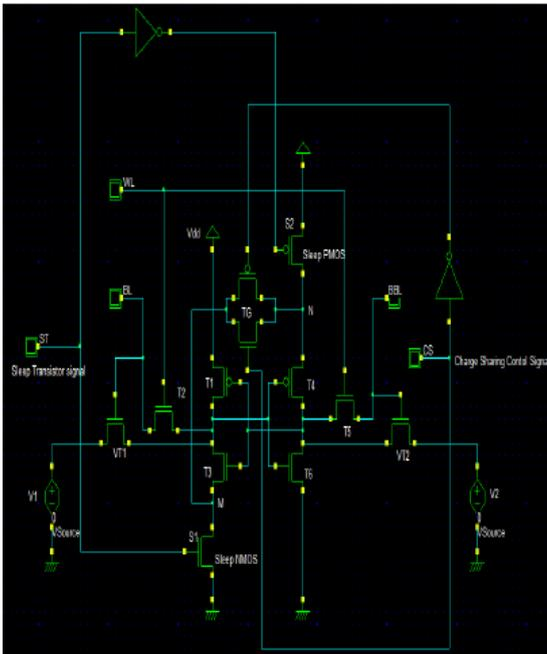
Fig5: 12T SRAM cell.
