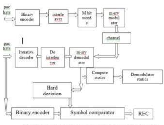
Figl:transmitter and receiver models with receiver statistics
