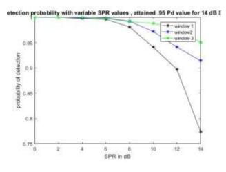
Fig7:probability of detection with variable SPR values
