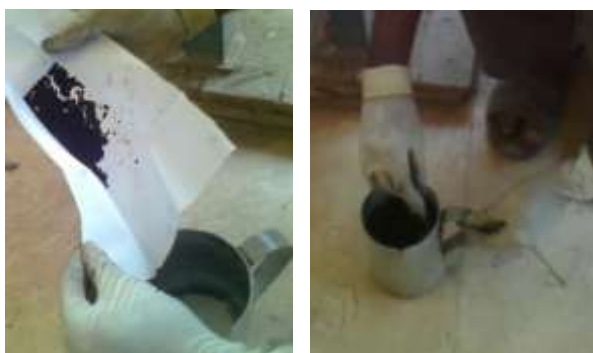
Fig. 4 adding and mixing of MWCNT into the mixture of polycarboxylate superplasticizer water solution
