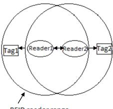
RFID reader range Fig.7. Reader-to-Reader Interference.
