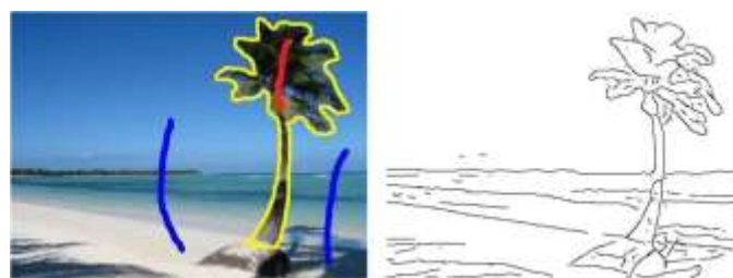
Fig. 1. (Left) Interactive image segmentation task with red and blue denoting seeds for the object and background. With the proposed framework, the whole palm tree can be cut out even when there is no seed at the trunk. (Right) Boundary map contains strong cues for segment labeling. We show how to fuse appearance and boundary information in segmentation. [7]
