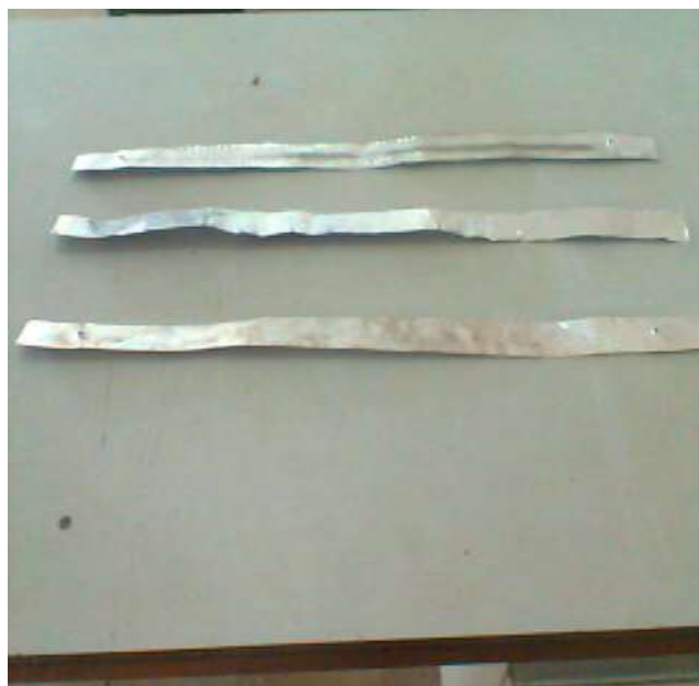
Plate 1(b): Specimens for the Foreign (China) Aluminum Roofing Sheets
