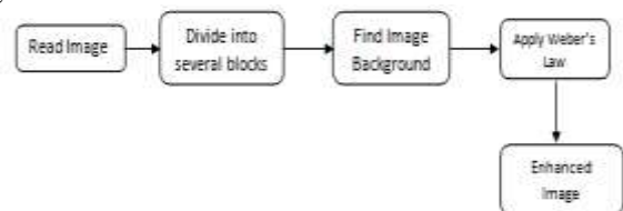
fig. 2.1.1 Block diagram of Background Detection by Block Analysis
