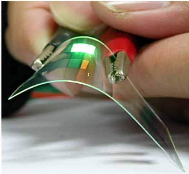
*Fig 1: Demonstration of flexible OLED device*
