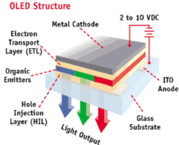
Fig 2: Structure of OLED
