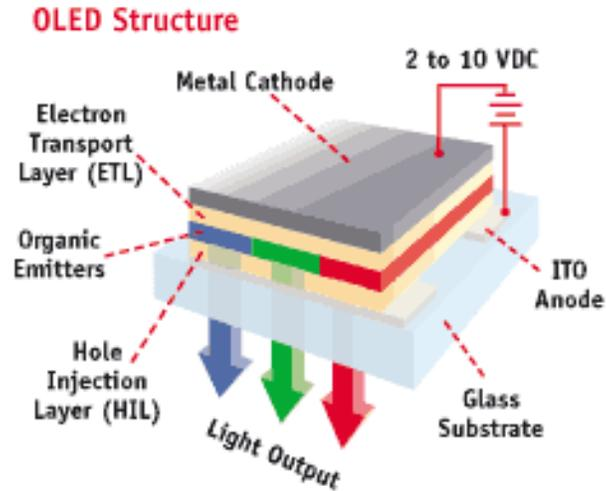
Fig 2: Structure of OLED
