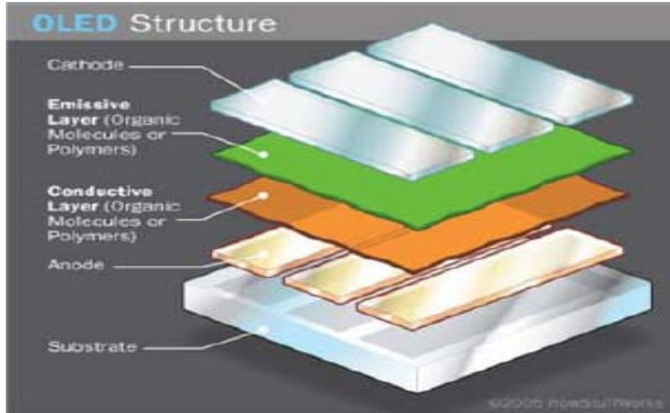
Fig 3: OLED Structure
