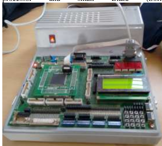
Fig 5. Experimental Setup of Object Tracking System Due to the advancement inside the fabrication technology and thus the rise inside the density of logic blocks on FPGA, the employment of FPGA is not restricted to any extent further to debugging and prototyping digital electronic circuits. As a results of the huge similarity realizable on FPGA and thus the increasing density of logic blocks, it's
