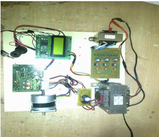
Figure.2. Circuit of BLDC Motor application (OFF state)
