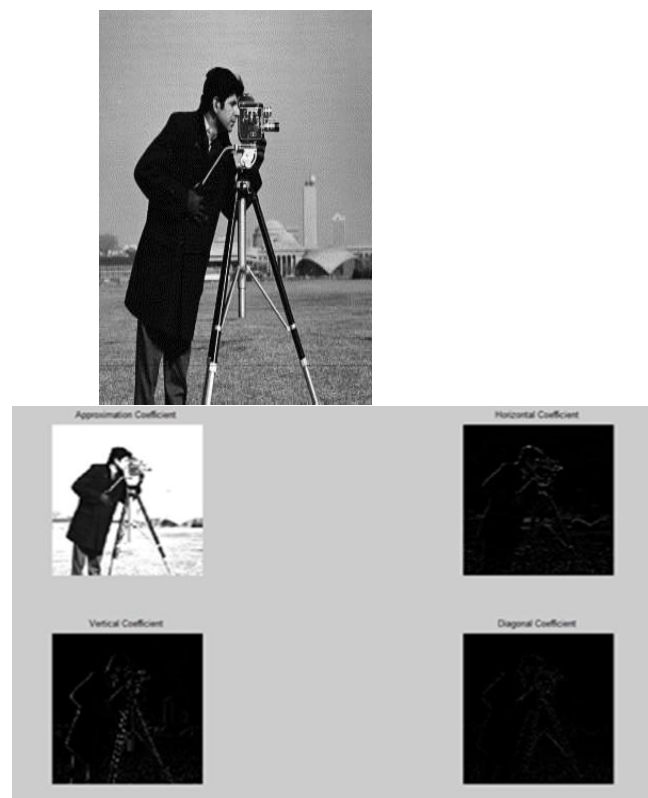
(a) Original Image (b) Image decomposition in approximate, vertical, horizontal, diagonal plane.
