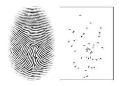
Figure 5: Grey scale fingerprint and extracted minutiae points
