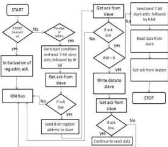
Fig-8 Flowchart for I 2 C master bus communication with slave device
