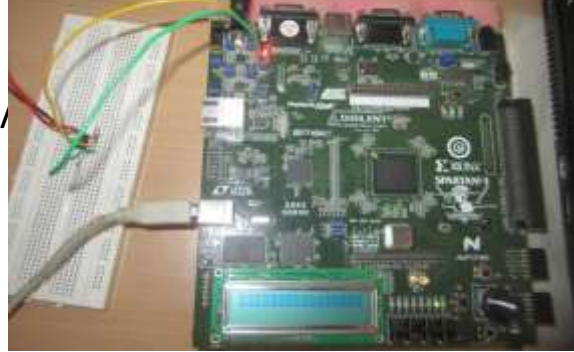
Fig-22 Hardware implementation in Spartan 3AN design kit
