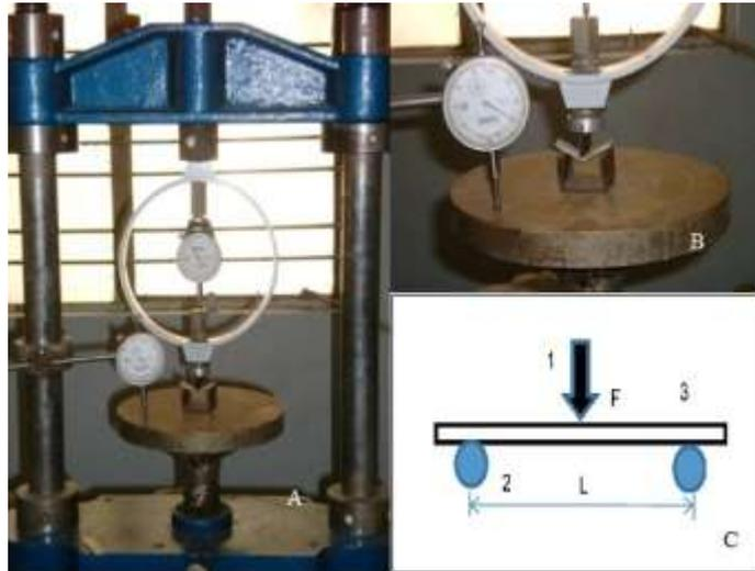
**Fig: Flexural Test Setup.**
