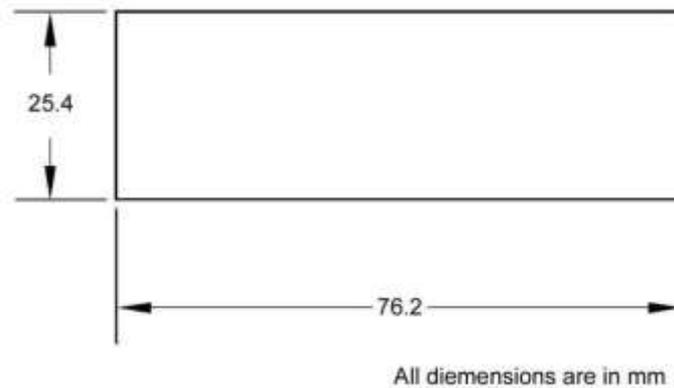
ASTM - D570 Water Absorption Test specimen Details.
