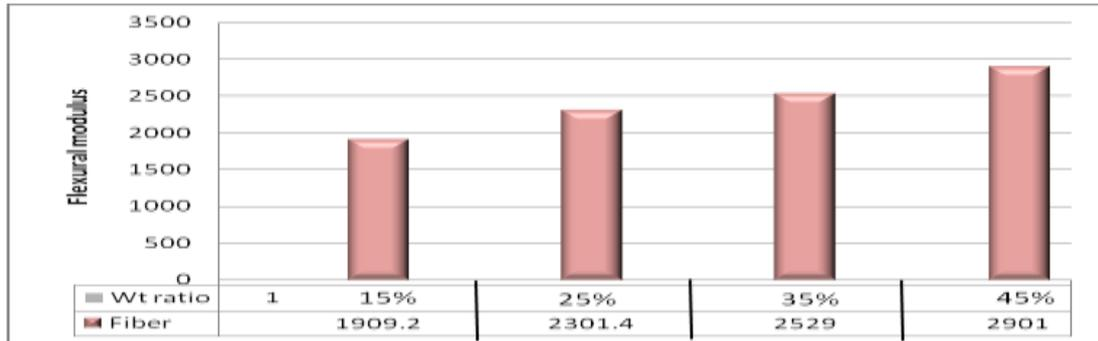
Fig.: Flexural Modulus for Different composites.
