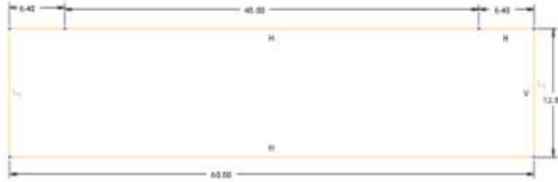
ASTM – D790 Flexural Test Specimen Details.
