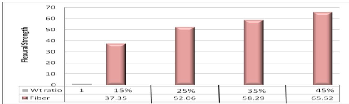
Fig: Flexural Strength for Different composites
