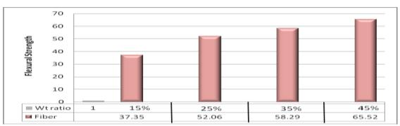
Fig: Flexural Strength for Different composites
