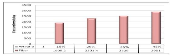
Fig.: Flexural Modulus for Different composites.
