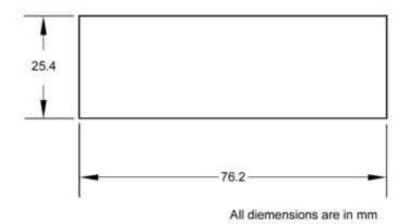
ASTM - D570 Water Absorption Test specimen Details.
