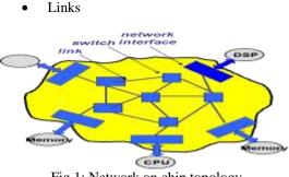
Fig 1: Network on chip topology
