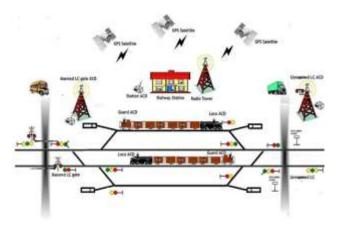
Fig.5.3:-Anti-collision device network
