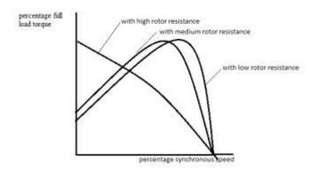
Fig:- Torque Versus Speed Characteristics
