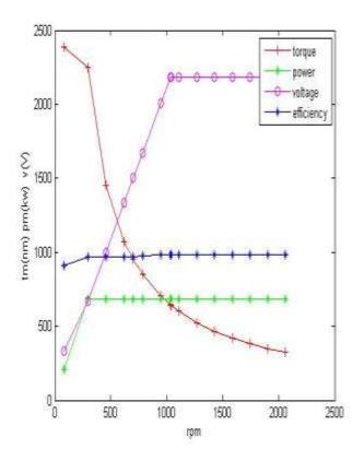
Ac Series Motor Output Charecteristics
