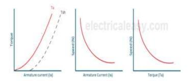
Note: ac series motor performance characteristics are slightly different from dc series motor
