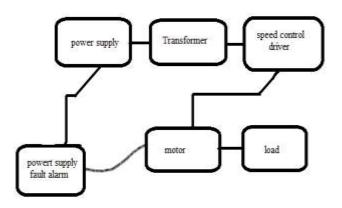
Fig: bi-direction speed control drive overview
