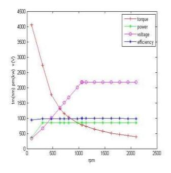
**3-Phase Induction Motor Output Characteristics**
