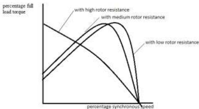
Fig:- Torque Versus Speed Characteristics
