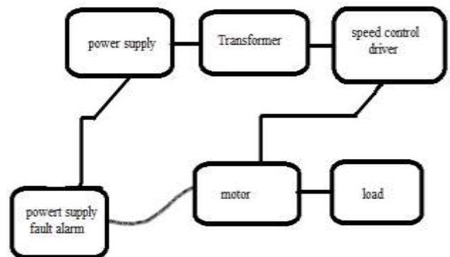
Fig: bi-direction speed control drive overview
