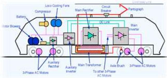
This is an example of "Power Conditioning" whose purpose is to provide pure DC or sine wave power free from harmonics or interference. Although it could be an integral part of a generator control system, more generally, power conditioning could also be provided by a separate free standing module operating on any power source.
