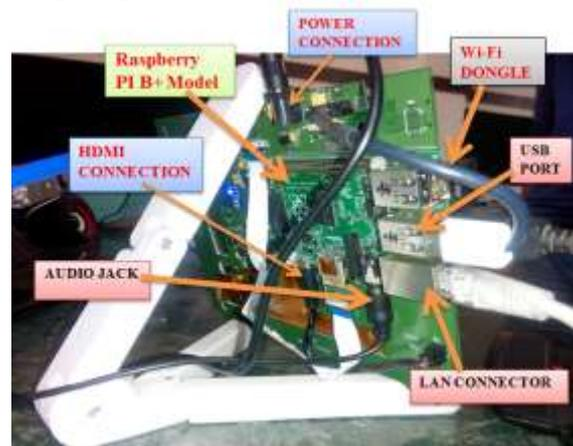
Figure 2.3: Connection setup of Raspberry Pi
