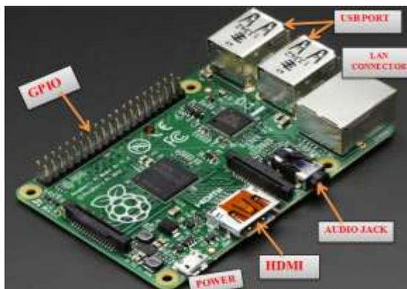
Figure 2.1: Raspberry Pi B+ model.
