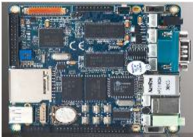
Fig.4: Mini2440 Development board
