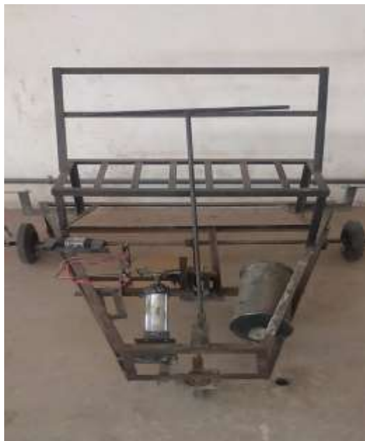
Fig. 2 Compressed air vehicle (assembled prototype)
