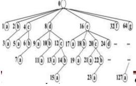
Fig.1. Reverse set enumeration tree where each node is numbered in the order of depth-first search.
