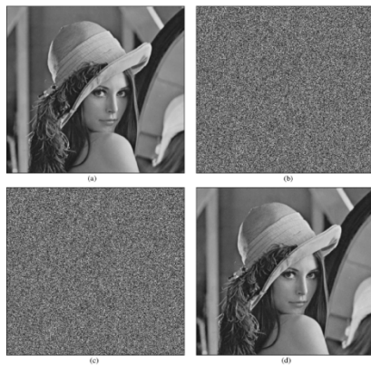
Fig. 3. (a) Original Lena, (b) its encrypted version, (c) encrypted image containing embedded data with embedding rate 0.017 bpp, and (d) directly decrypted version with PSNR 39.0 dB.
