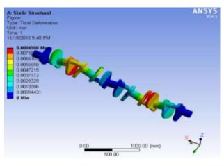
Figure 15. Total deformation in steel
