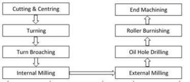
Figure 6. Machining process for manufacturing crankshaft
