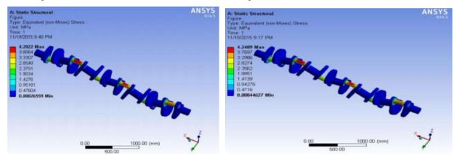
Figure 17. Von-Mises stress in steel
