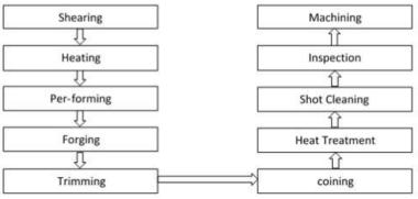
Figure 4. Forging process for manufacturing crankshaft
