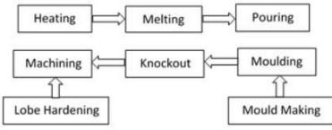
Figure 5. Casting process for manufacturing crankshaft
