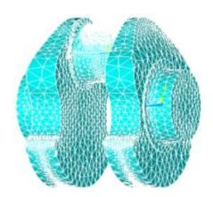
Figure 22. Meshed model of crankthrow
