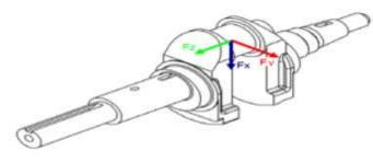
Crankshaft geometry and bending ( $F_x$ ), torsional ( $F_y$ ), and longitudinal ( $F_z$ ) force directions
