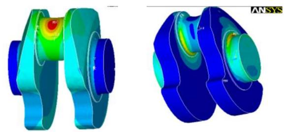
Figure 25. Total deformation in crankthrow Figure 26. Von-Mises stress in crankthrow The 3-D model of the entire crankshaft was prepared using Pro/Engineer software and meshed in ANSYS software.
