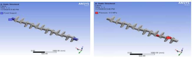
Figure 13. Boundary conditions Figure 14. Loading of 3.5N/mm<sup>2</sup> Von-Mises stress and total displacement values were determined applying structural steel and Inconel X-750 as the materials, using static structural analysis as shown in Fig. 15, Fig.16, Fig. 17 and Fig. 18 respectively for structural steel and Inconel-X750.
