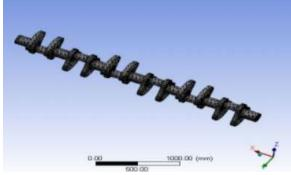
Figure 11. Crankshaft model
