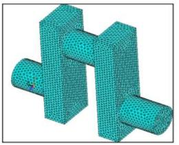
Figure 28. Meshed model in ANSYS
