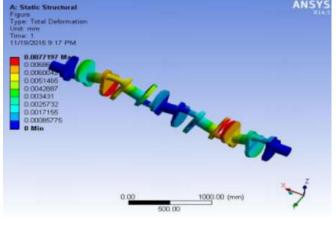
Figure 16. Total deformation in Inconel X-750
