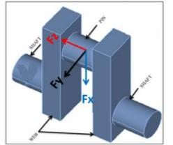
Figure 27. Crankshaft model in CATIA
