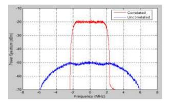
Figure 5 (a) Output Spectrum of a Nonlinearity Partitioned into Correlated and Uncorrelated Components; Reverse Link 5 DPCH
