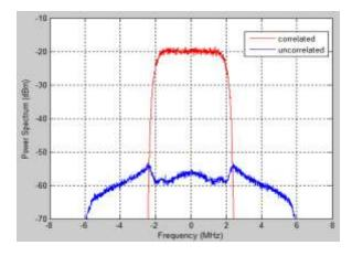
Figure 2 (a) Output Spectrum of a Nonlinearity Partitioned into Correlated and Uncorrelated Components; Forward Link 1 DPCH
