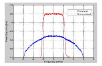
Figure 4 (a) Output Spectrum of a Nonlinearity Partitioned into Correlated and Uncorrelated Components; Forward Link 16 DPCH
