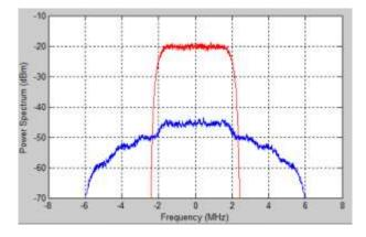
Figure 3 (a) Output Spectrum of a Nonlinearity Partitioned into Correlated and Uncorrelated Components; Forward Link 3 DPCH
