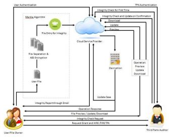
Fig. 2. System architecture Diagram
