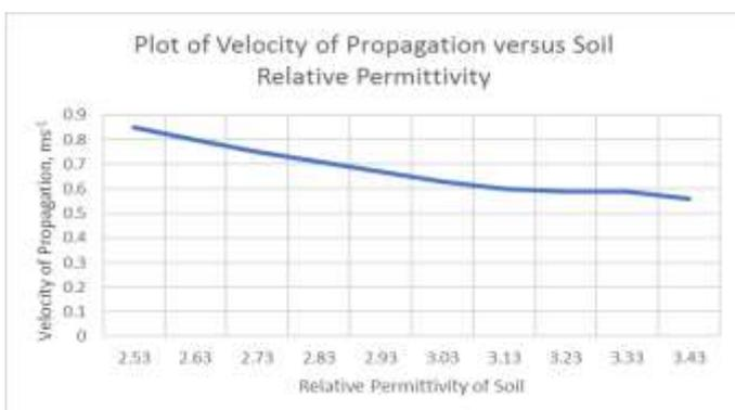
**Figure 7:** Plot of velocity of propagation (fractional) against soil relative permittivity
