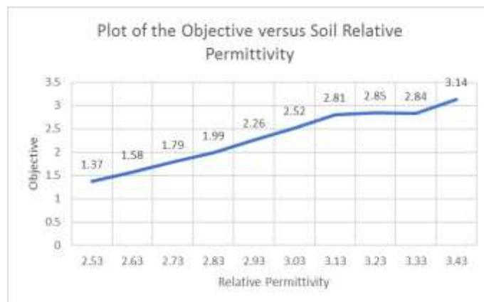
**Figure 2:** Plot of the objective with changing soil relative permittivity
