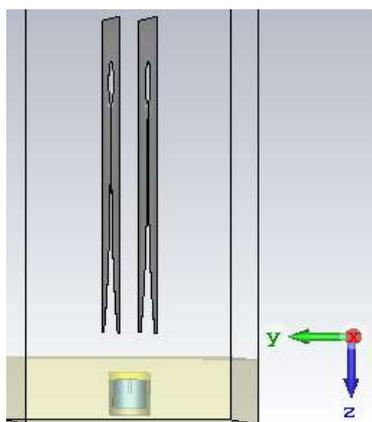
**Figure 1:** Bistatic Vivaldi handheld GPR system model
