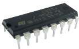
Fig.6. L293D motor driver
