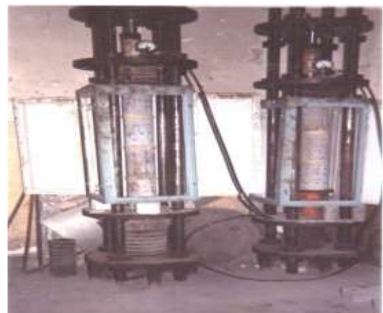
Fig. 3- Test specimens in creep loading frame
