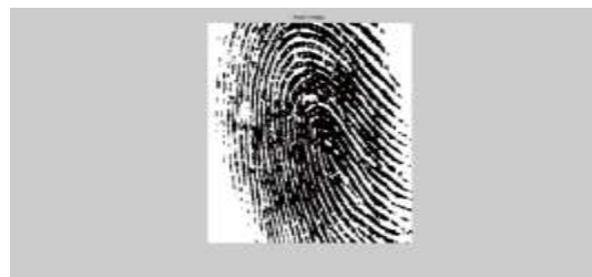
Fig: Output obtained after the binarization of the fingerprint impression.
