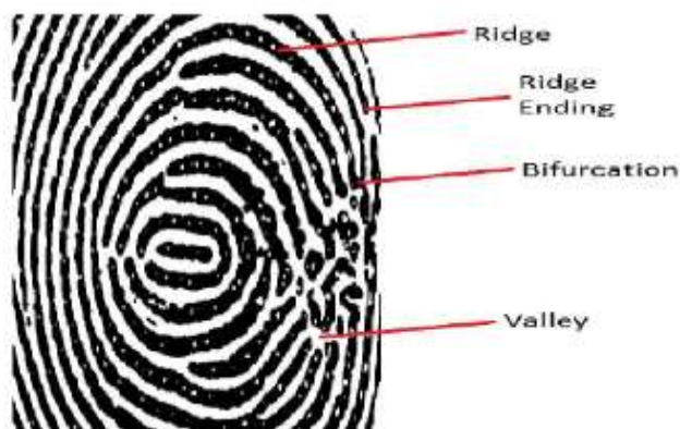
Fig: Minutiae points in Fingerprint
