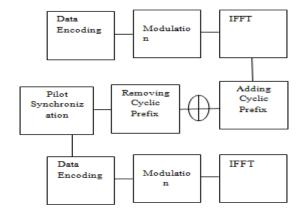
Figure 3.3: OFDM system transmitter and receiver section based on DFT
