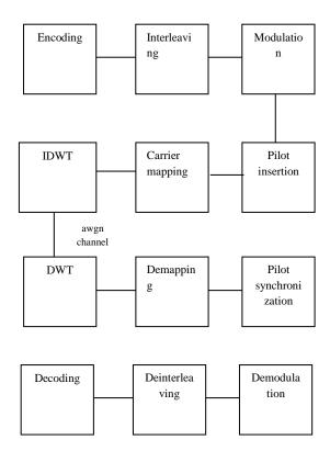
Figure 3.5: Design system model of wavelet based OFDM
