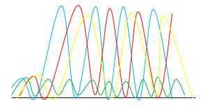
**Figure 1:** Orthogonality in orthogonal frequency division multiplexing (OFDM)
