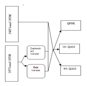
Figure 4.1: DFT and DWT based OFDM with various modulation techniques
