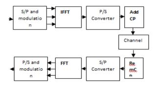
Figure 2: Block diagram of Basic OFDM system
