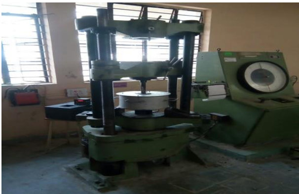
Fig. 13 Hot Extrusion Setup
