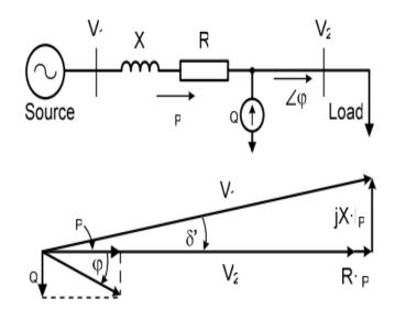
Fig. 4 system with compensation in shunt
