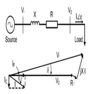
Fig. 5 system without compensation in series
