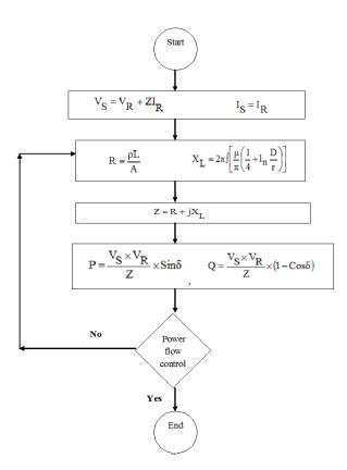
Fig. 2 flow chart for Solution domain
