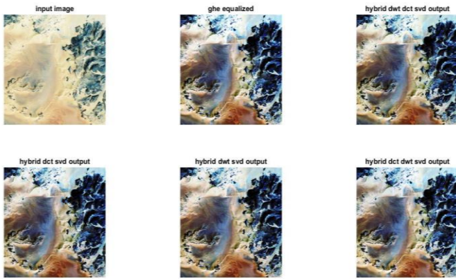
Fig-12: Input Image and Improved Images by using GHE, DWT-DCT-SVD, DCT-SVD, DWT-SVD AND DCT-DWT-SVD for Image 7
