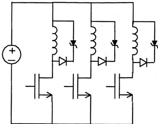
Fig. 2. Simple unipolar converter for three-phase BLDC motor.
