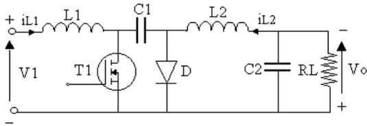
Fig. 5. Circuit diagram of CUK converter
