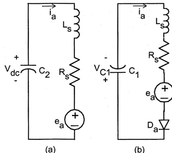
Fig. 4. Equivalent circuits of each machine phase when (a) the switch is on and (b) when the diode is conducting
