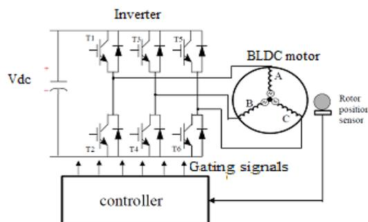
Fig. 1. Basic BLDC motor control system with position sensors.
