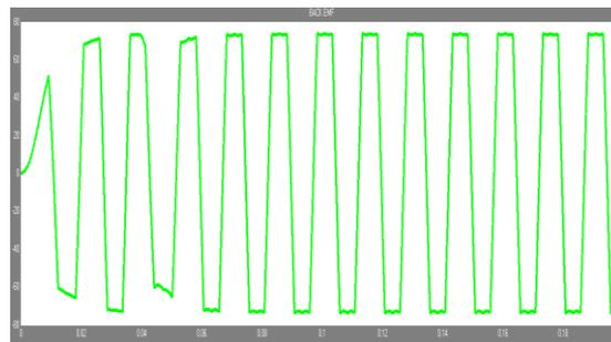
Fig. 9. Back emf waveform of one phases
