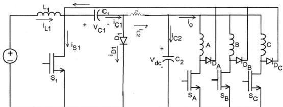
Fig. 3. Schematic of CUK converter based BLDC motor drive.
