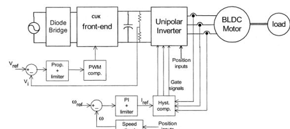
Fig. 6. Block diagram of the drive system.
