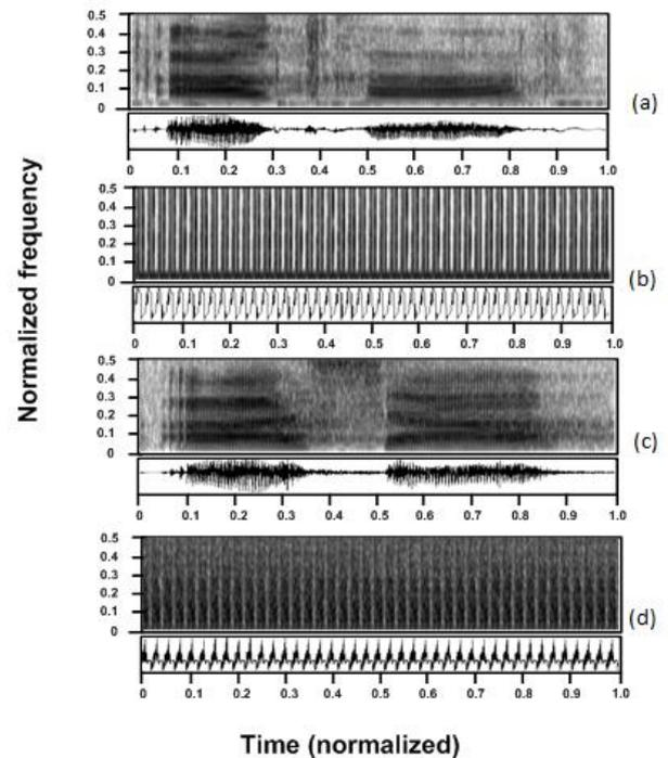
**Figure 11:** Spectrogram of aspirated consonant (a) Original speech signal (आखा) (b) Facial EMG signal (आखा) (c) Original speech signal (आँख) (d) Facial EMG signal (आँख) for Sp6.
