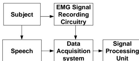
**Figure 5:** Block diagram for EMG signal acquisition.
