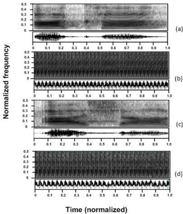
**Figure 9:** Spectrogram of aspirated consonant (a) Original speech signal (आखा) (b) Facial EMG signal (आखा) (c) Original speech signal (आँख) (d) Facial EMG signal (आँख) for Sp4.
