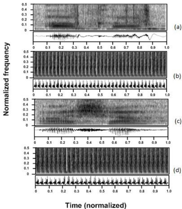
**Figure 6:** Spectrogram of aspirated consonant (a) Original speech signal (आखा) (b) Facial EMG signal (आखा) (c) Original speech signal (आछा) (d) Facial EMG signal (आछा) for Sp1.
