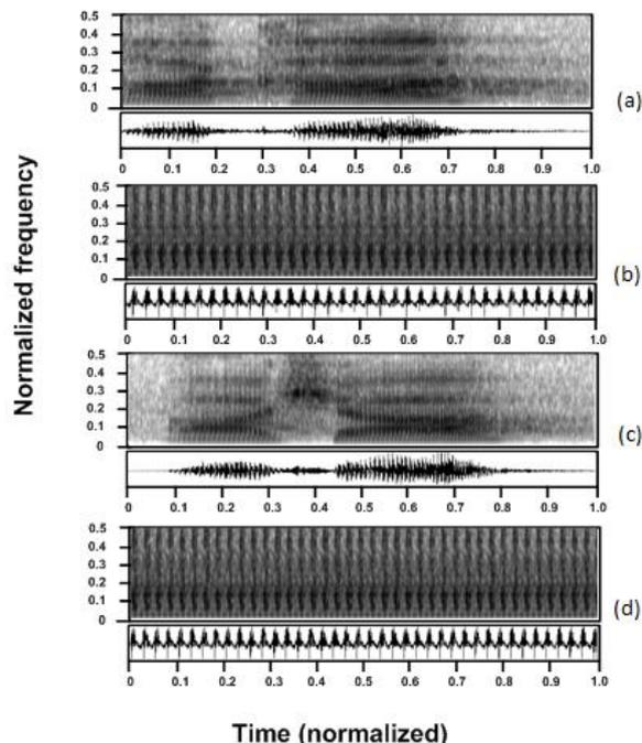
**Figure 7:** Spectrogram of aspirated consonant (a) Original speech signal (आखा) (b) Facial EMG signal (आखा) (c) Original speech signal (आछा) (d) Facial EMG signal (आछा) for Sp2.
