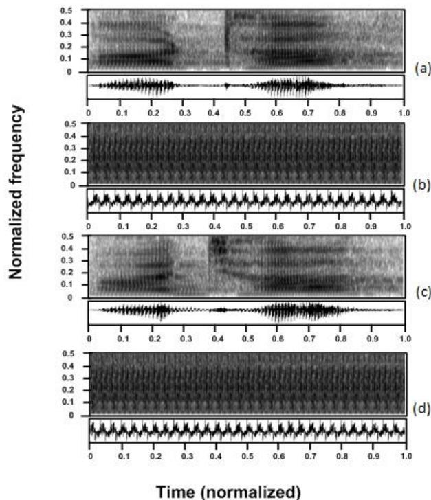
**Figure 8:** Spectrogram of aspirated consonant (a) Original speech signal (आखा) (b) Facial EMG signal (आखा) (c) Original speech signal (आछा) (d) Facial EMG signal (आछा) for Sp3.
