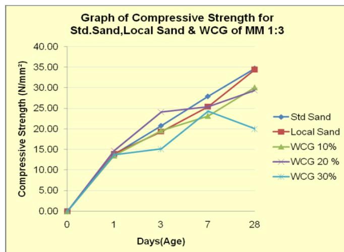
**Figure 4:** White coarse glass compressive strength result
