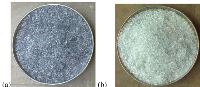
**Figure 1:** Photo of material used (a) Colour coarse glass aggregate (b) White coarse glass aggregate
