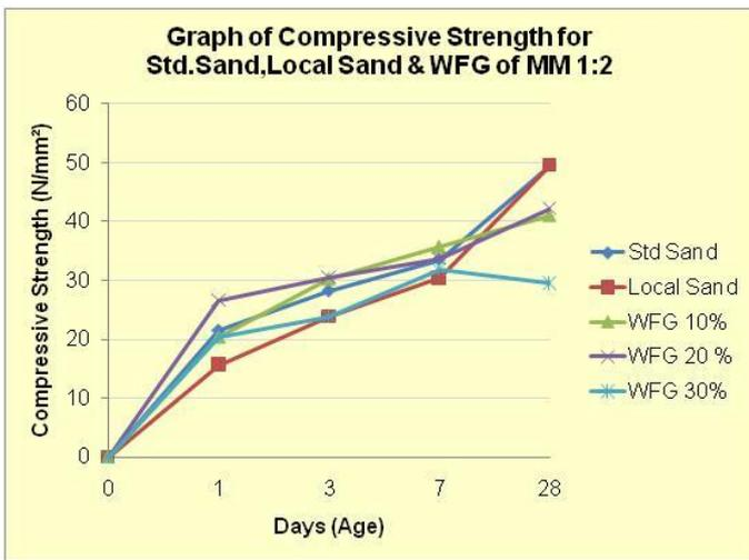
Figure 5: White fine glass compressive strength result
