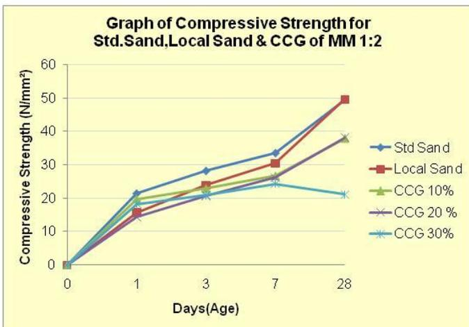
Figure 6: Colour coarse glass compressive strength result
