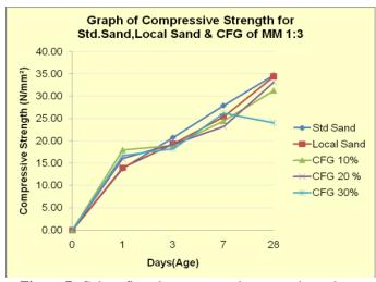
Figure 7: Colour fine glass compressive strength result
