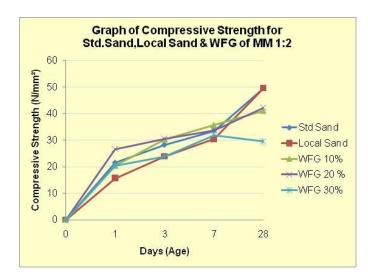
Figure 5: White fine glass compressive strength result
