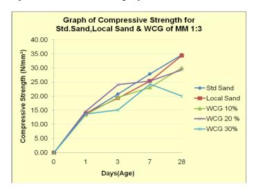
Figure 4: White coarse glass compressive strength result
