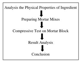
Figure 2: Flow Chart of Experimental Work
