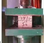
**Figure 3:** Picture of sample testing (a) Specimen before testing (b) Specimen after testing
