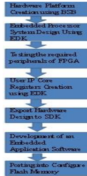
Fig. 3. Configuration of Embedded System Processor
