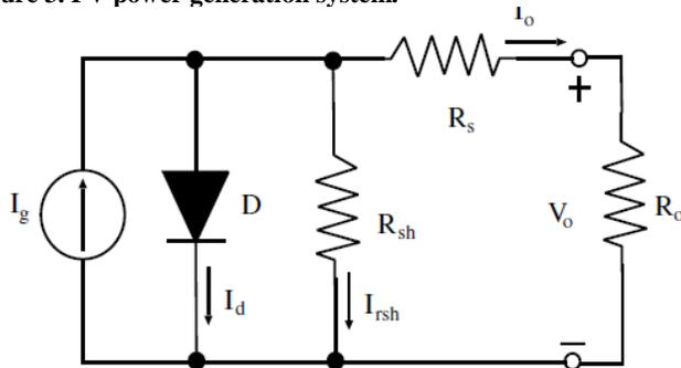
Figure 4. Equivalent circuit of a solar module.
