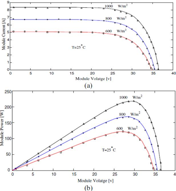
Figure . Solar module characteristic curves. (a) Current-voltage curves. (b) Power –voltage curves. The discrete data points shown are taken from the manufacturer’s curves [15], and show excellent correspondence with the model.
