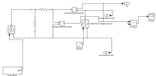
Pv cell equivalent diagram in simulation
