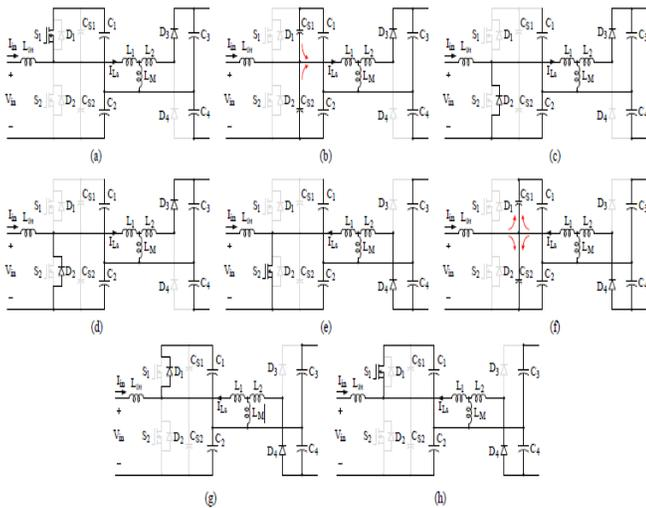
Commutation step diagrams during a switching cycle
