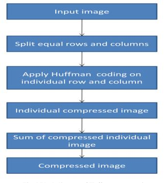
Fig. 1 Block diagram of Huffman compression
